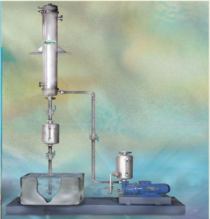
SUCTION PRESSURE: 67 TORR. DESIGNED FOR A DRY NUTSEEDS & SNACKS PLANT
